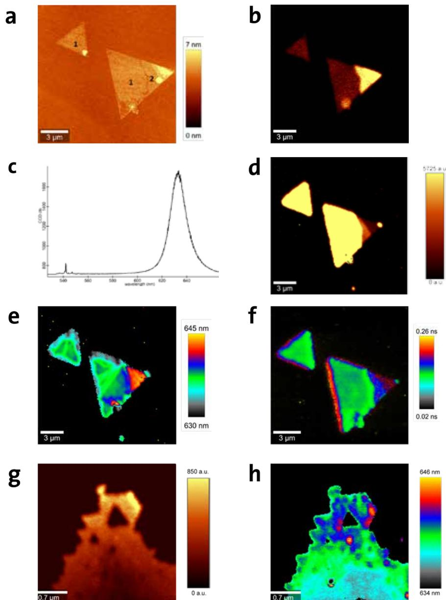
Fig. 3: Correlative AFM-SNOM-PL imaging of WS<sub>2</sub>
