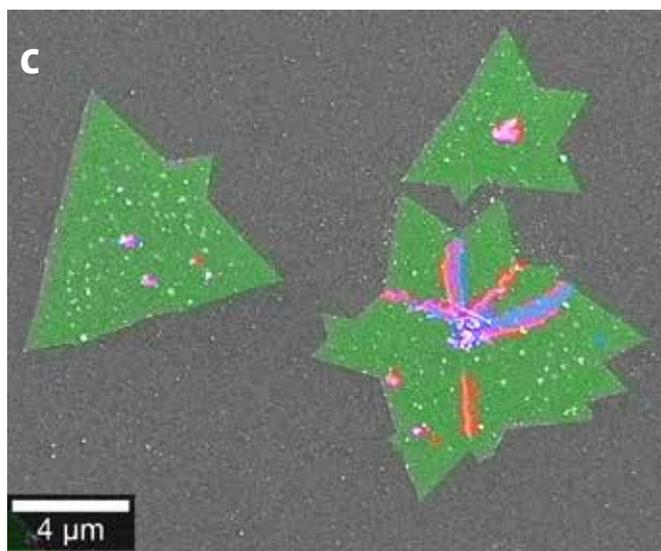
Fig. 2: RISE microscopy of MoS<sub>2</sub> crystals
