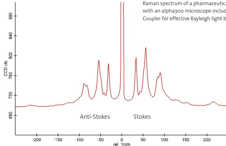
Raman spectrum of a pharmaceutical sample acquired with an alpha300 microscope including the RayShield Coupler for effective Rayleigh light blocking.
