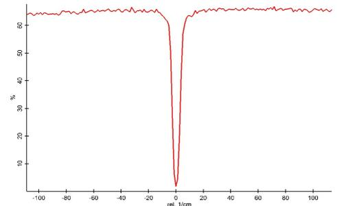
The graph above shows the extremely high transmission rate (in percentage) for Stokes and Anti-Stokes signals at wavenumbers down to 10 rel.  $\text{cm}^{-1}$ .
